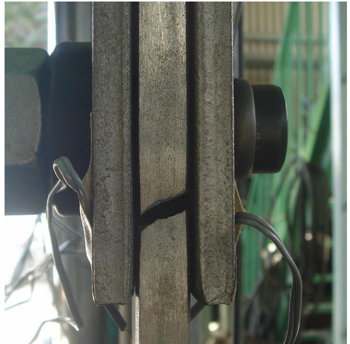
Photograph 6. Fracture of base material (M3)
